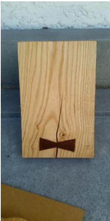
Incrustation assemblage papillon
